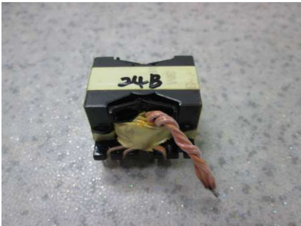
Overall view of transformer
