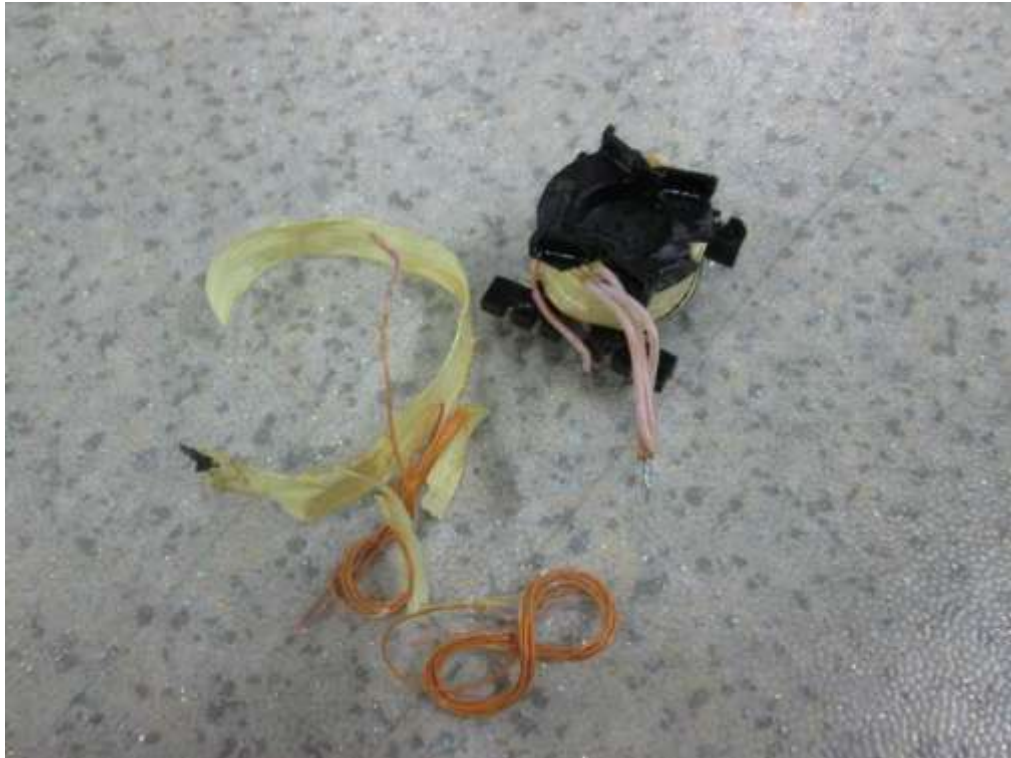
Internal view of transformer
