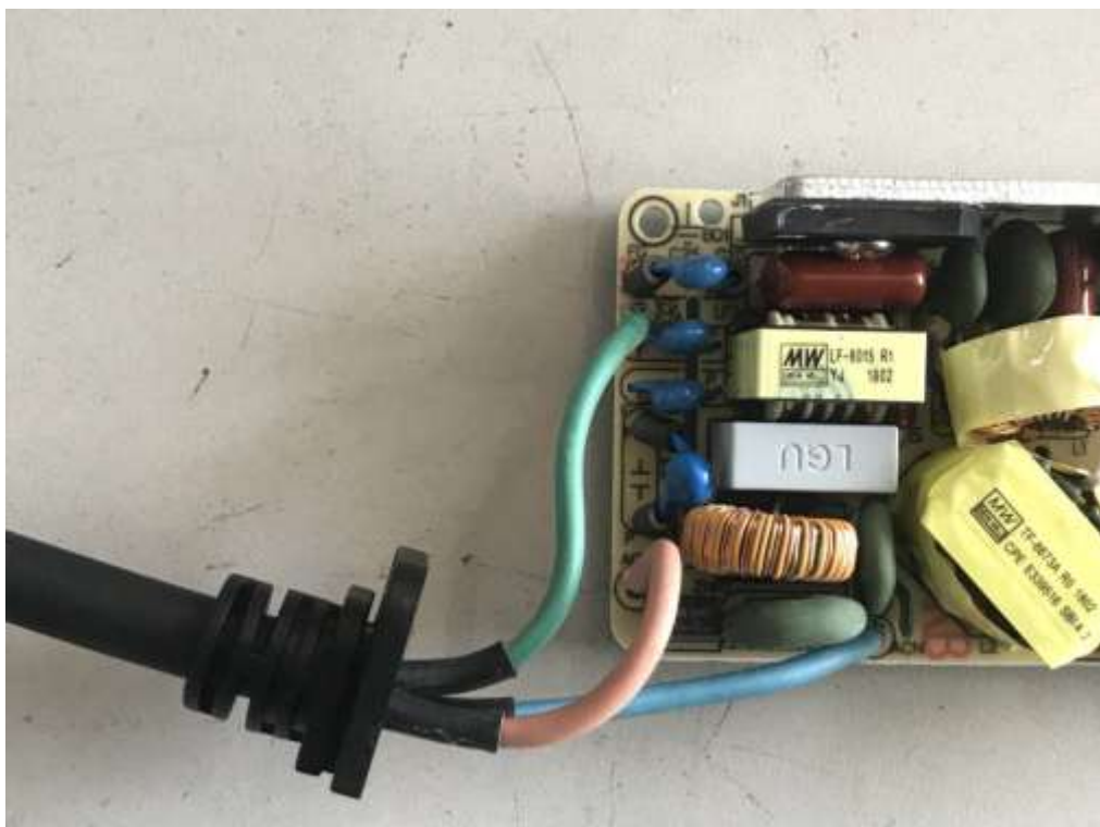
Alternative earthing construction view on PCB board (fixed by soldering)
