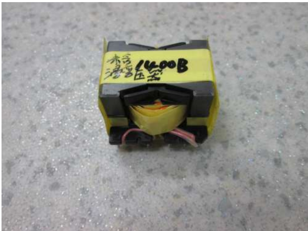
Overall view of transformer
