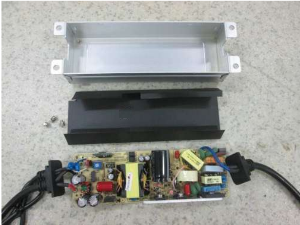
Internal view, ELG-100-C1400B before potting
