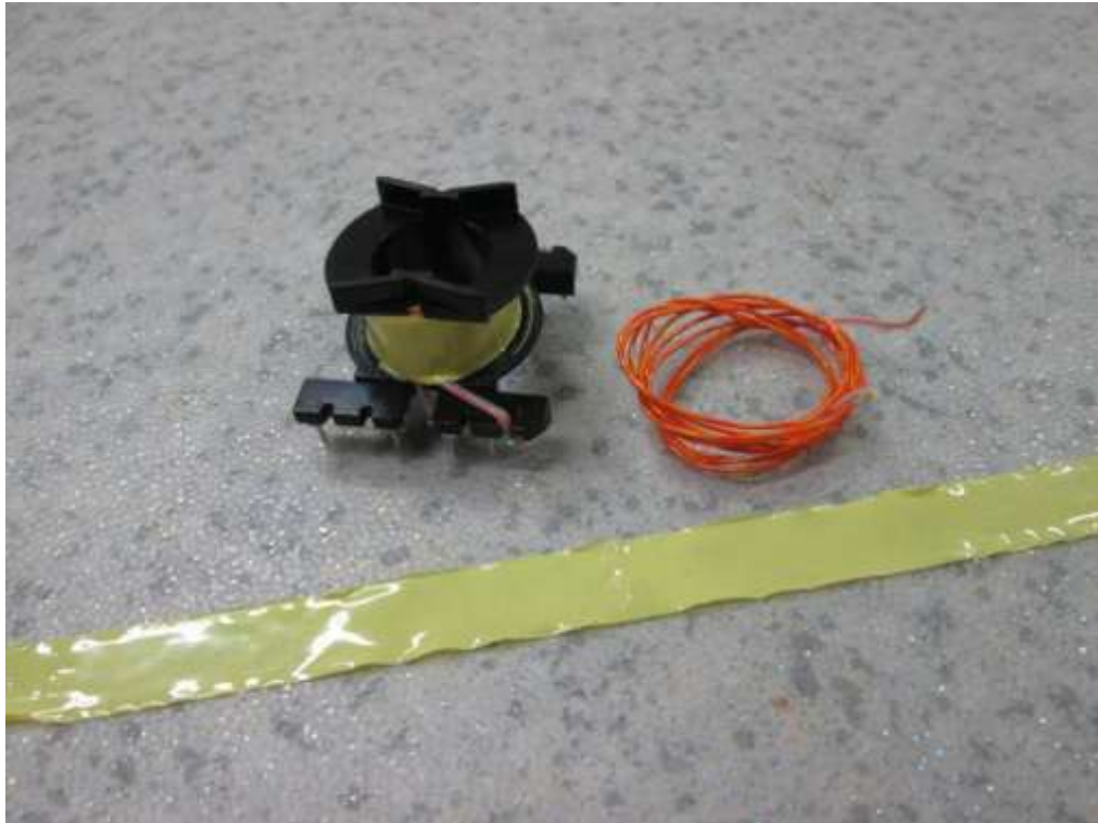
Internal view of transformer
