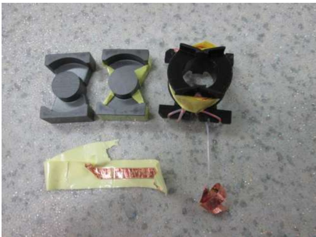
Internal view of transformer
