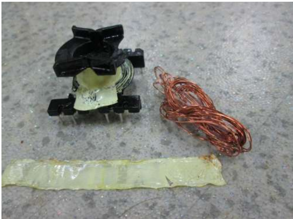
Internal view of transformer
