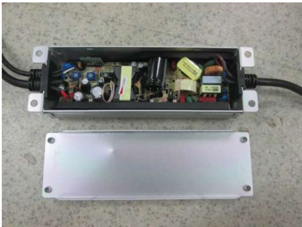
Internal view, ELG-100-54B before potting
