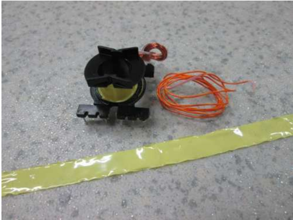
Internal view of transformer
