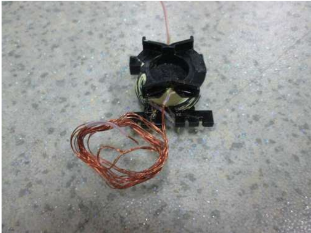
Internal view of transformer
