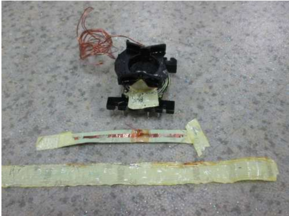
Internal view of transformer
