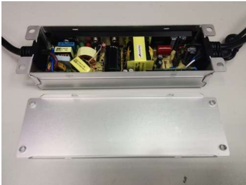
Internal view, ELG-100-C1400DA before potting
