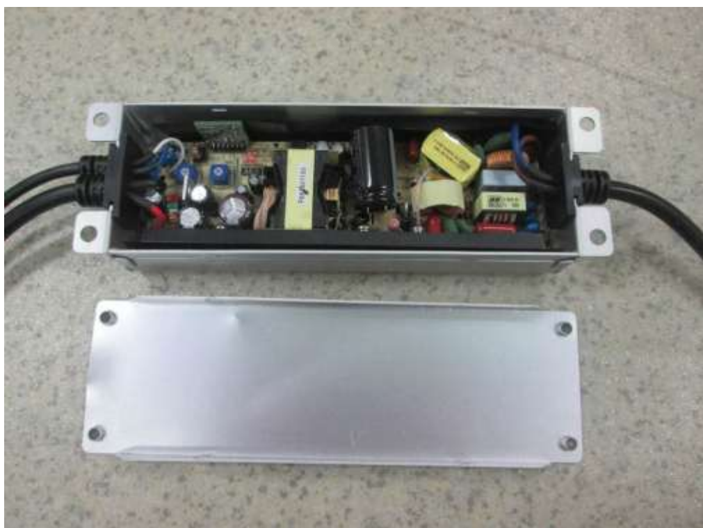
Internal view, ELG-100-24B before potting
