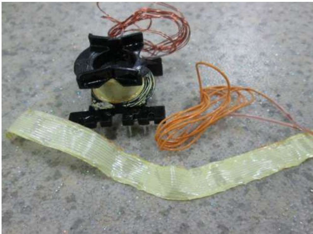
Internal view of transformer
