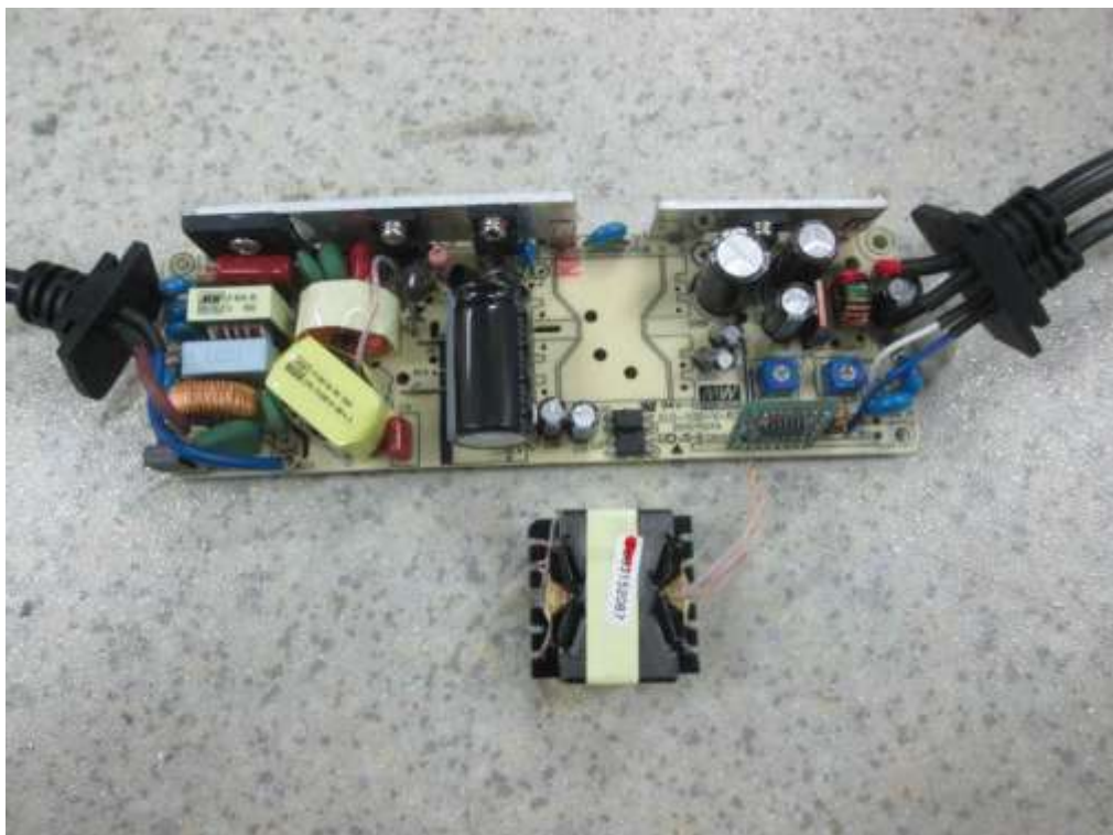
Internal view after transformer removed
