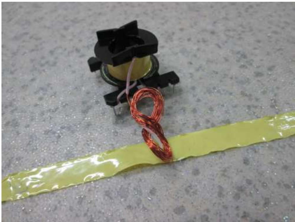
Internal view of transformer
