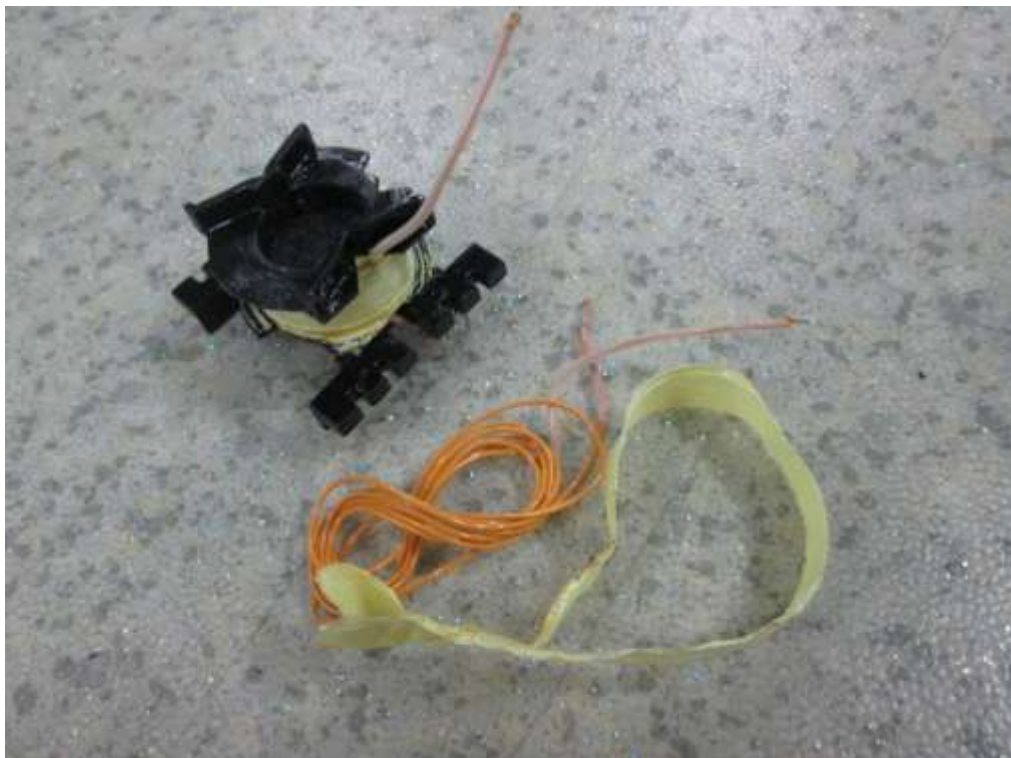
Internal view of transformer
