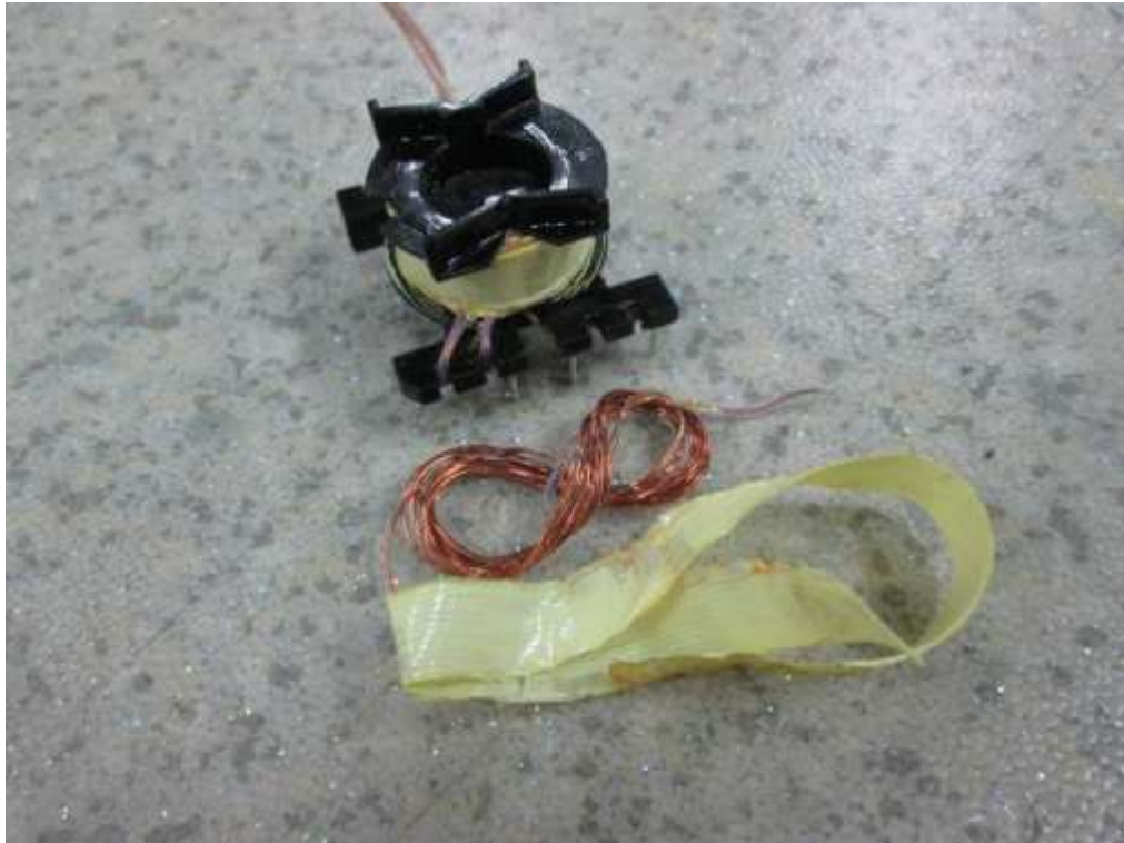
Internal view of transformer
