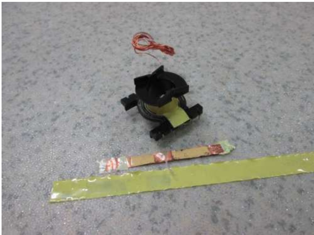
Internal view of transformer
