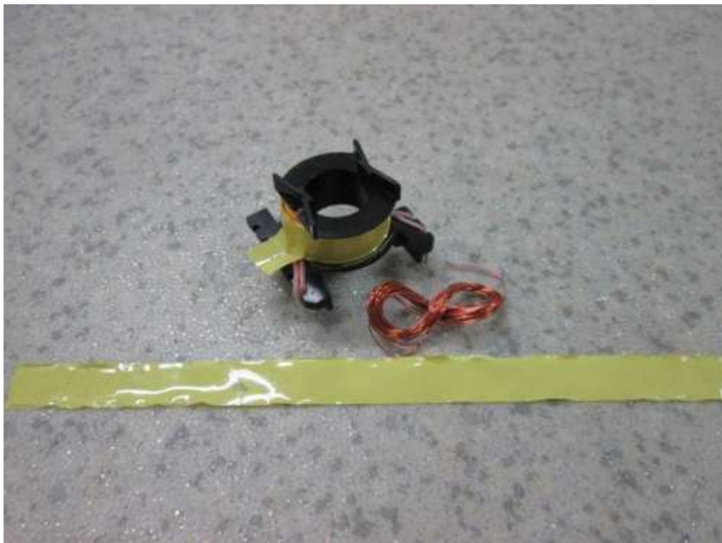
Internal view of transformer
