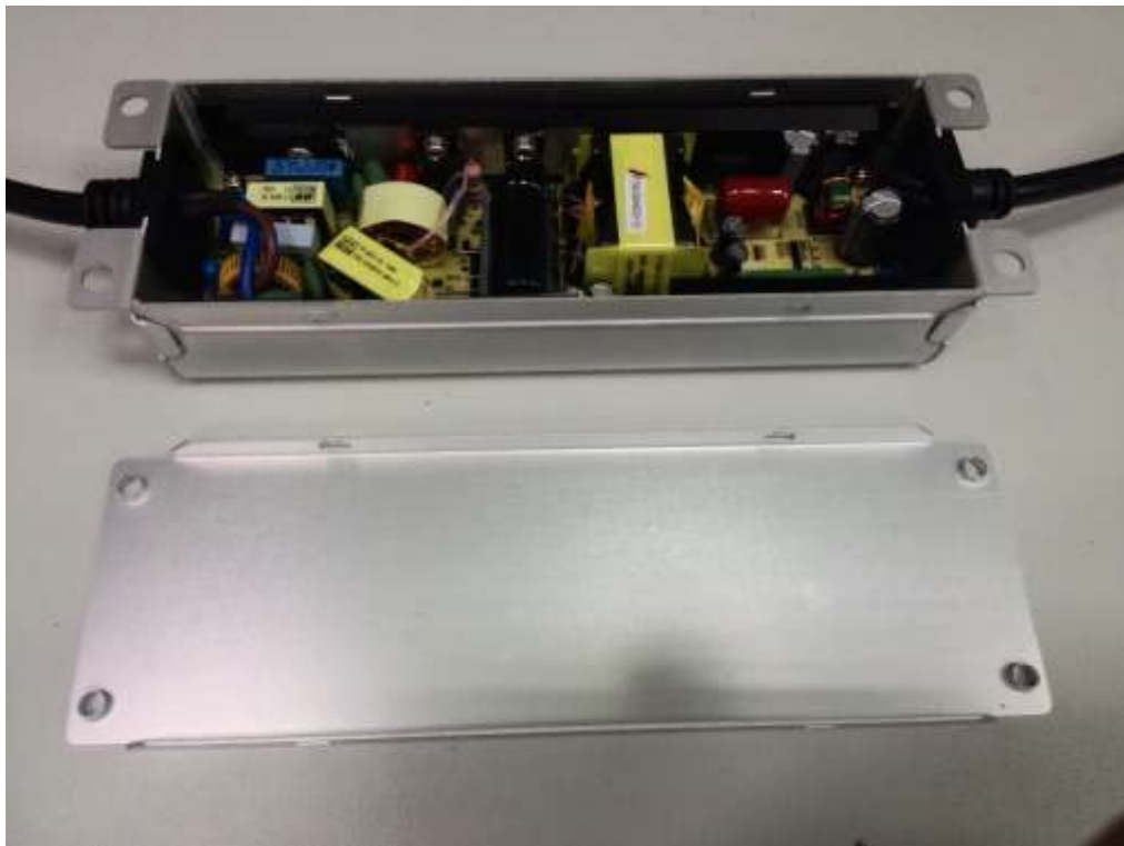
Internal view, ELG-100-C1400D before potting
