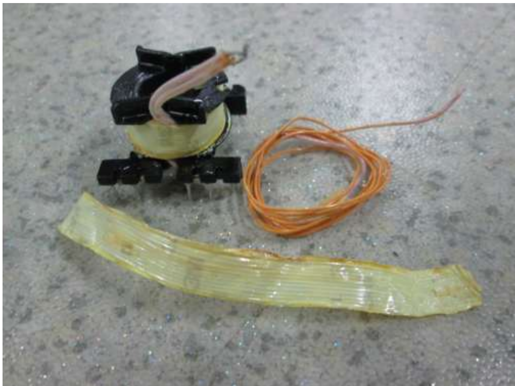
Internal view of transformer
