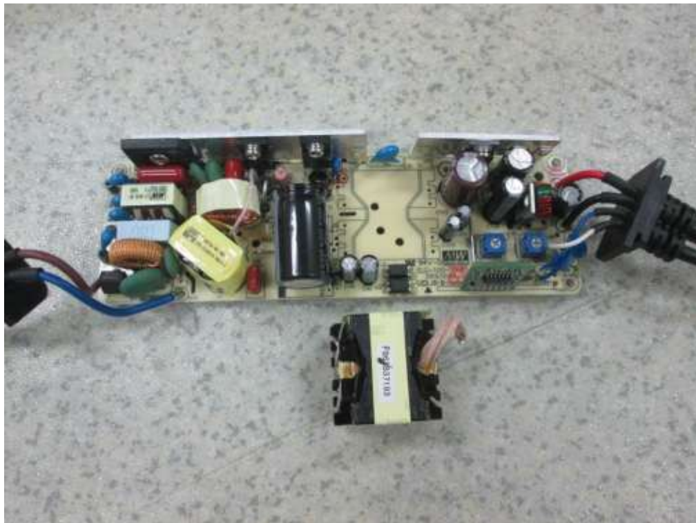
Internal view after transformer removed
